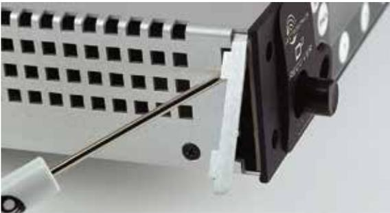
3. Insert the flange bracket (Part #27076) into the open slot in the side of the chassis cover panel.
