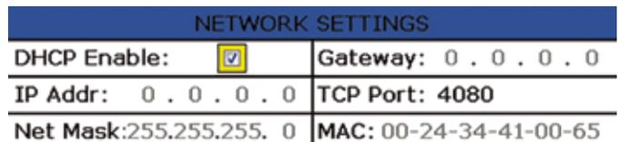
NOTE: New network settings require the unit to reboot to take effect. Making a change and pressing the BACK key will prompt the user to Reboot Now, Save and Exit, or Discard and Exit.
