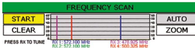
**NOTE:** All four channels scan at the same time. You can also select individual channels for scanning by pressing the channel selector buttons.
