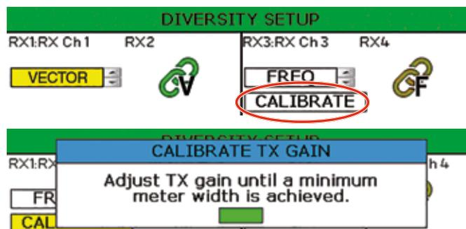
4. Adjust the microphone gain on each transmitter to balance the audio level while observing the green bar on the screen. When audio level is balanced, the green bar is minimized.
