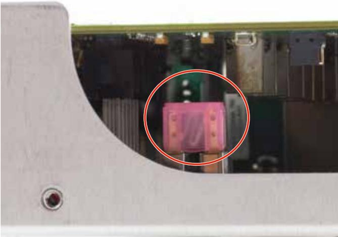
This is a standard 4A, 32VDC mini blade (automotive type) fuse. You can obtain one from any automotive or electrical supply shop, or order one from us (part #21941). Replace if necessary.
