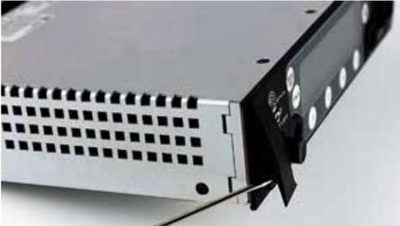
2. Remove the breakaway tabs on both sides of the chassis side panels. Use a flat blade screwdriver to pry the tabs outward and snap them off of the chassis.
