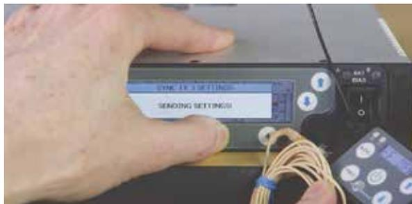
**NOTE:** You must position the transmitter's IR port directly in front of the DSQD IR port, as closely as possible, to guarantee a successful sync. A message will appear on the DSQD if the sync was successful or failed.
