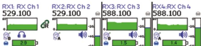
**Choose Transmitter:** Choose one of four Rx channels by using the **Channel Selector Buttons**, 1, 2, 3 or 4. Hold and press the Channel Selector Button to initiate sync.
