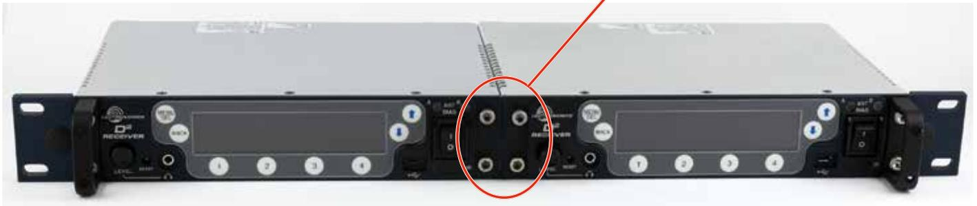
7. Remove the four cap screws from the adjacent rear panels, and then use them to attach the rear tie bracket. Do not tighten the screws completely.
