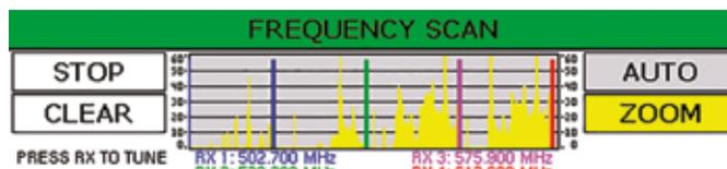
3. Press one of the four channel selector buttons. The word **TUNING** will flash on the screen to let you know you are tuning. Press the **UP** and **DOWN** arrows to tune the channel into the area of lowest RF activity.
