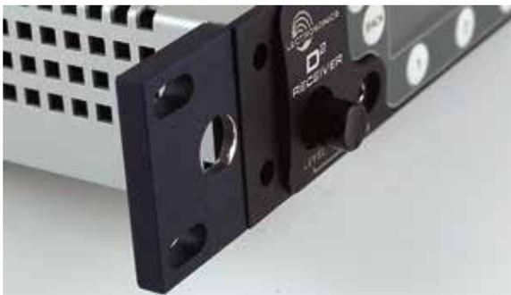
4. Insert two (2) cap screws (Part #28885) through the rack handle (Part #27082) holes and install the rack handle onto the flange bracket through the holes in the unit's front panel. Firmly tighten the cap screws using the hex key (Allen wrench) as shown.
