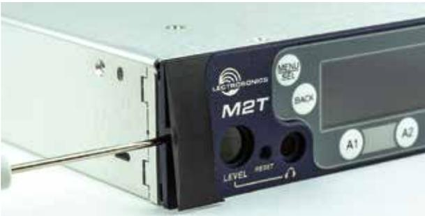
2. Remove the breakaway tabs on both sides of the Chassis Cover Panel. This requires the use of a flat-blade screwdriver inserted into the slots and levering the tabs away on each side of the unit.
