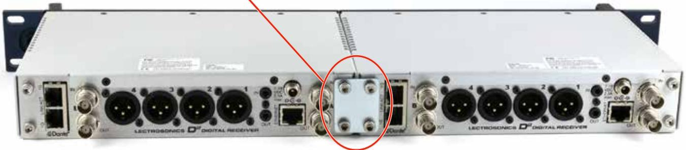
8. After front and rear tie brackets are installed, place the receivers on a flat surface so that the front panels are even with each other. Hold the receivers in place and tighten all cap screws on the front and rear brackets.
