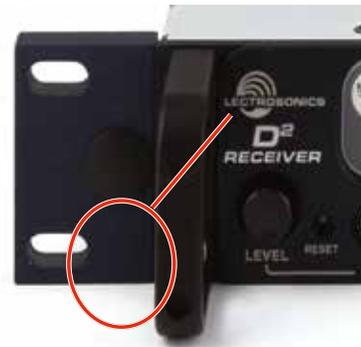
**NOTE:** The retaining nuts on the panel and tie brackets are “tensioning lock nut” types designed to prevent the screws from coming loose due to vibration. You will usually feel resistance as you tighten the screws - this is normal.
