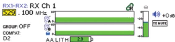
**NOTE:** Press and holding channel selector buttons will initiate a sync with a transmitter from most screens.
