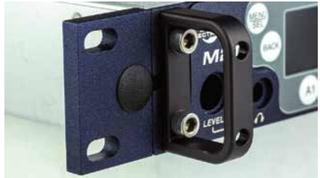
6. Install the Front Tie Bracket (Part #25991) into the open slot in the right side of the M2T Chassis Cover Panel with the protruding nuts facing rearward, affix with two (2) Cap Screws (Part #28885) provided and firmly tighten with the Hex Wrench. See next page.
