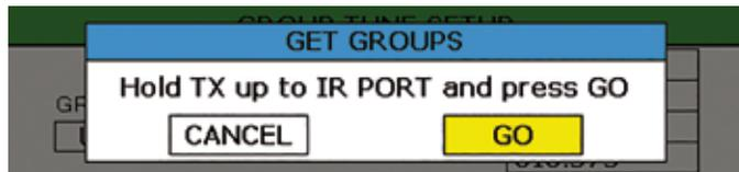
When a tuning group is assigned, the frequency control is limited to the frequencies contained in the tuning group. It also limits the available frequencies in the frequency coordination process.
