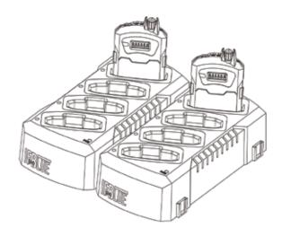
Use only rechargeable NiMH batteries and set the battery selector switch in the IFBR1C to NiMH, as shown.
